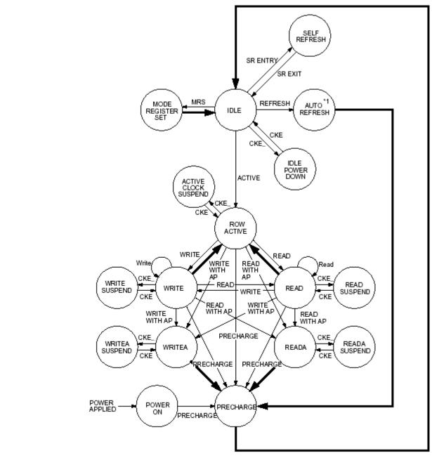
Automatic transition after completion of command.
